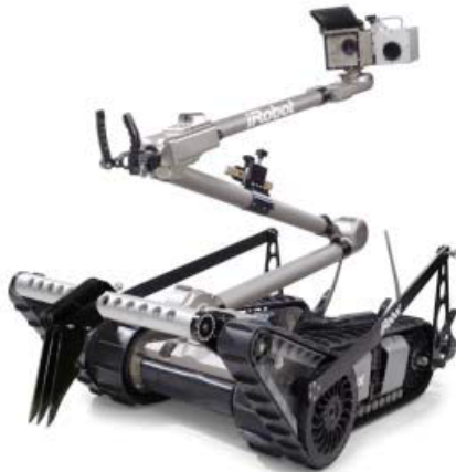
Figure: PackBot: a military mobile robot.
