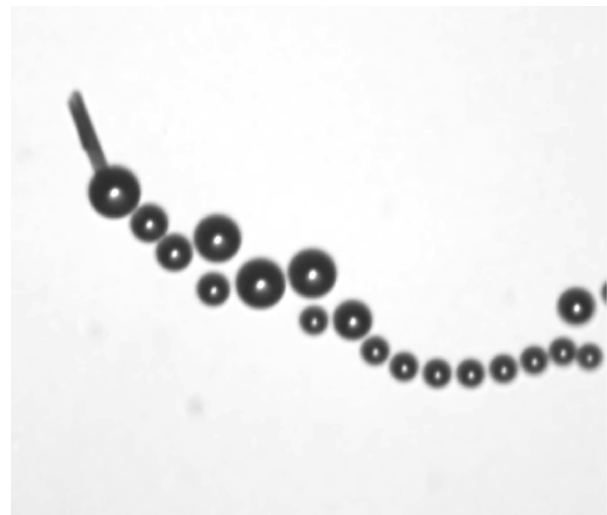
Figure 1. Ti/Fe/Pt rolled-up microtubes achieve self-propulsion in hydrogen peroxide solution [1]. The catalytic decomposition of the solution into water and oxygen bubbles. The bubbles provide thrust force and enable self-propulsion, whereas the iron layer of the microtube enables directional control under the influence of external fields.
