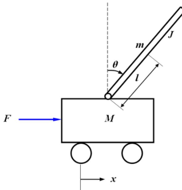
Figure 1: The cart-pendulum system.
