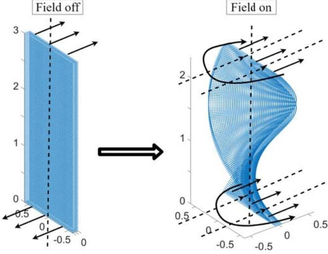
Figure 1: MagTwist, with the longitudinal axis, magnetic field lines (dotted arrows) and polarity direction (solid line arrows)
