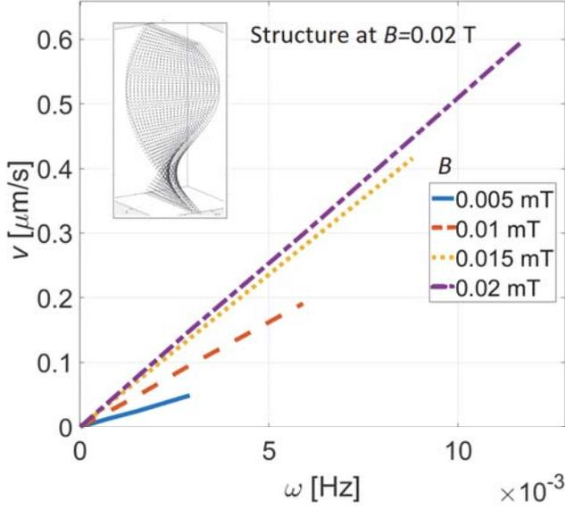
Figure 11: Velocity of MagTwist for varying magnetic field strength, plotted against the rotation frequency at viscosity = 3.18 Pas
