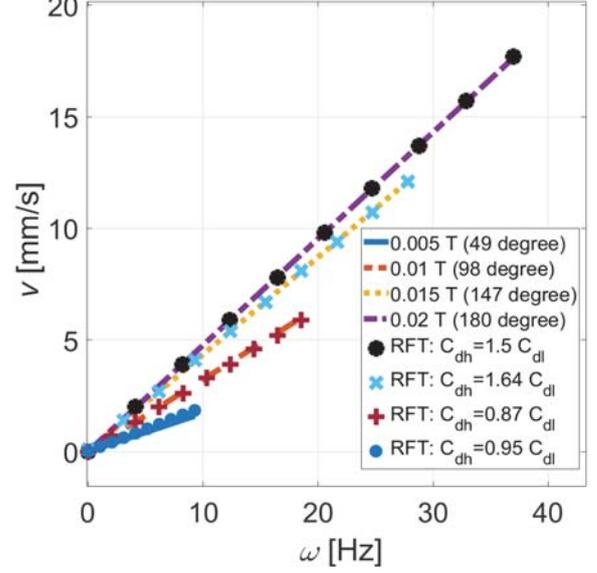
Figure 12: Velocity of MagTwist for varying magnetic field strength, plotted against the rotation frequency at viscosity = 0.001 Pas, compared with RFT model
