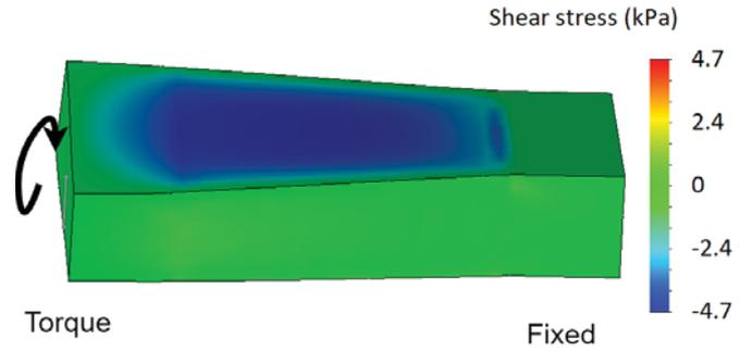
Figure 10: Stress analysis in Solidworks with torque boundary condition on left magnetic part and clamped boundary condition on the right magnetic part
