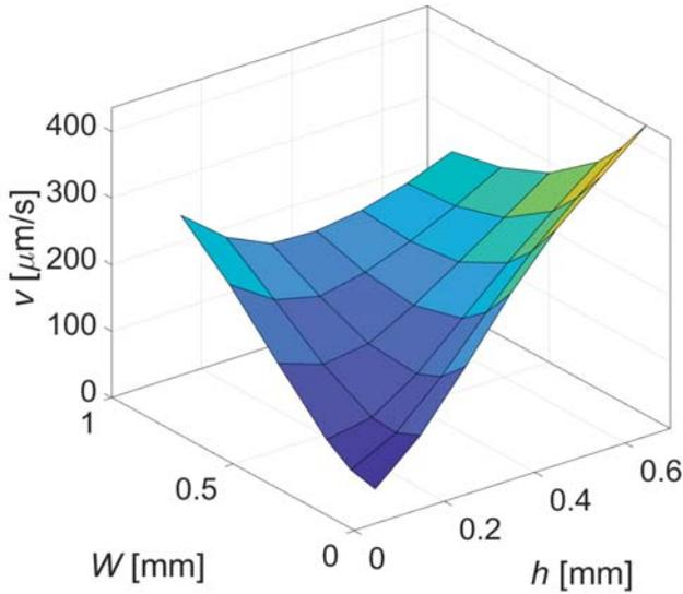
Figure 5: Varying width and thickness. The height/width ratio should be large to maximise velocity
