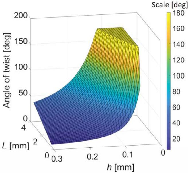
Figure 8: Angle of twist for varying length and thickness
