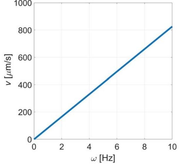
Figure 4: The linear velocity of MagTwist increases with the angular velocity linearly below the step-out frequency.
