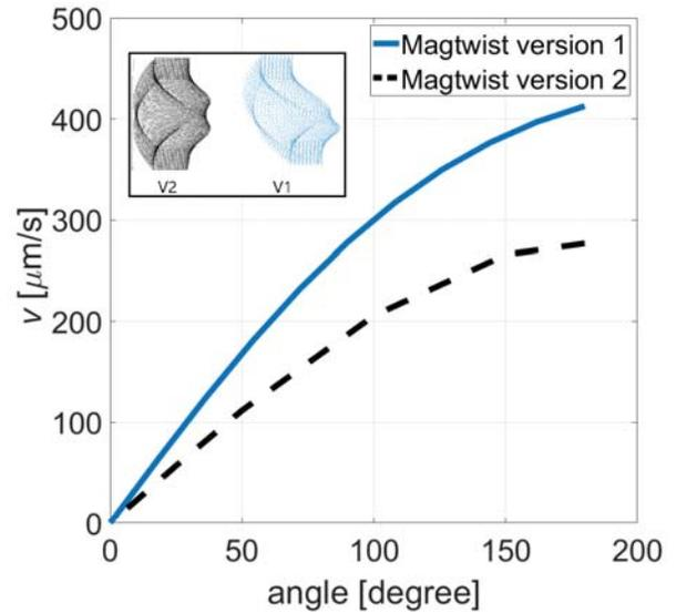
Figure 7: The swimming velocity for MagTwist version one and two at different angle of twists ( $\omega = 5$  Hz)
