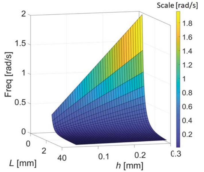
Figure 9: Cut-off frequency for varying length and thickness
