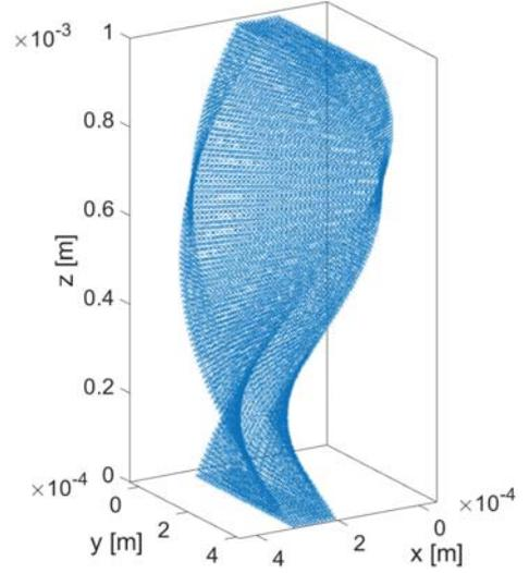
Figure 2: MagTwist is represented using a distribution of Stokeslets boundary points. The deformation of MagTwist about the z-axis is characterized by the angle of twist ( $\pi$ ).
